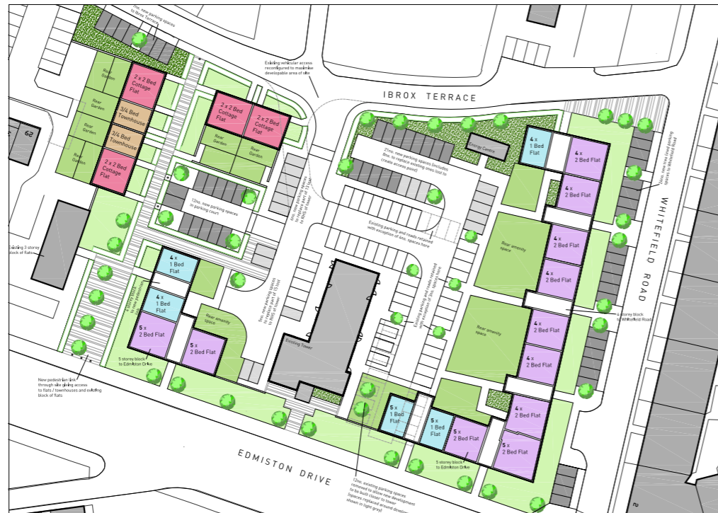
1. Above: Initial Proposals with continuous perimeter block plus parking to Whitefield Road, blocks within site on Ibrox Terrace
